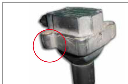
Crack formation on the ignition coil insulation due to strain during installation.
