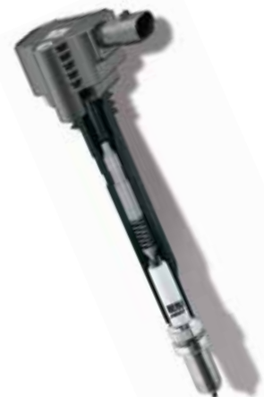
Space-saving and highly efficient BERU ignition system: double platinum spark plug with Plug-Top ignition coil. The internal pressure spring 'bowl' connector on the new double platinum spark plug prevents insulator flashovers.
