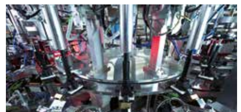
One of the most important steps in the production sequence: final inspection of the ignition coil.
