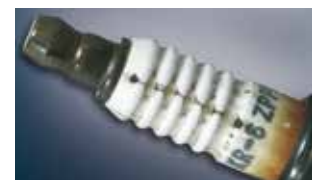
Scorch marks on the spark plug neck – a sign of misfiring.
