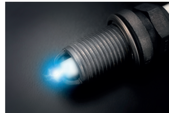
Each spark plug delivers non-stop sparks between around 500 and 3500 times a minute.
